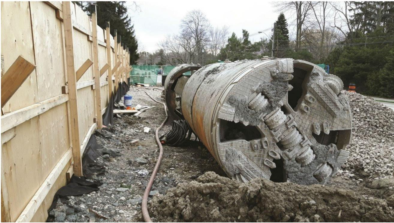
The microtunnel drives were located up to 14 metres below ground surface and excavated with an MTBM on a grade of approximately 0.15 percent.
